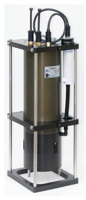
The optional deployment cage provides protection for the a-Sphere and pump during deployment and handling, while still providing access to the sphere for cleaning.
